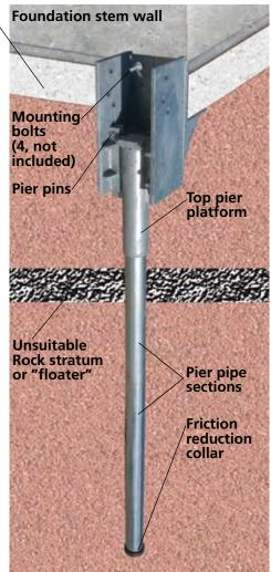
Pre-Drilled Plate Bracket Atlas Resistance® Pier Systems also are available by special order with capacities matching those listed below. See page 5 for general information on Plate Bracket Systems.
